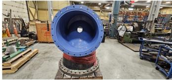
Belzona 1341 for coating inside the surface
