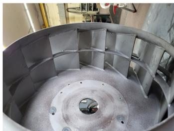
Blasted fan with 1311 reinforcing welds and filling holes and pits
