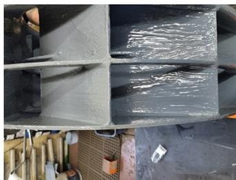
2 coats of 1321 on inside and all fins + welds. 2 colors as a wear indicator for inspection
