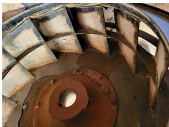
Worn blower, about half way through its usual lifespan, makeshift balancing bolts.
