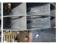
2 coats of 1321 on inside and all fins + welds. 2 colors as a wear indicator for inspection
