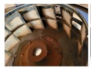
Worn blower, about half way through its usual lifespan, makeshift balancing bolts.
