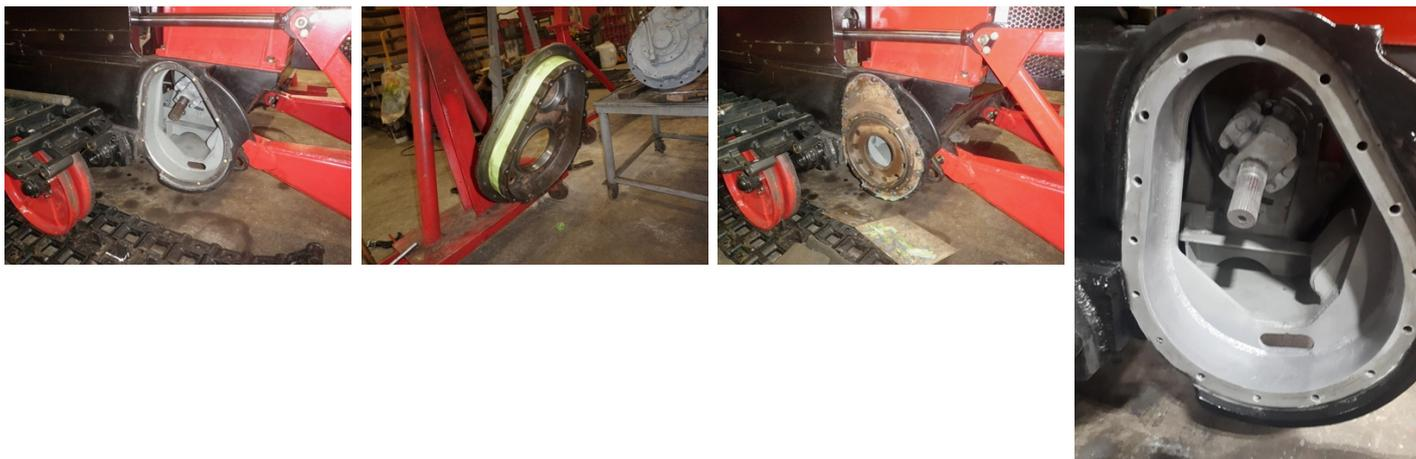
The final drive housing seat is not damaged, but it is out of alignment due to frame distortion. The mating surface will be cleaned and prepped with a mechanical blaster and all bolt holes corked, then Belzona 1111 will be applied over it.
