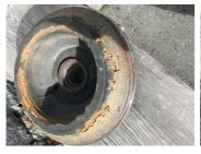
This pump casing was extremely corroded and eroded corrosion and erosion creating an unacceptable efficiency.
