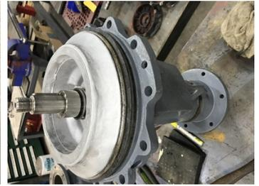
This pump casing was extremely corroded and eroded creating an unacceptable efficiency.
