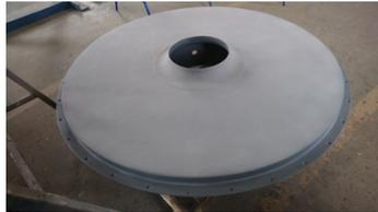
In terms of cleaning the cover from acids, it was necessary to wash and blast the cover several times.
