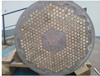
The repair was done using cork plugs.
