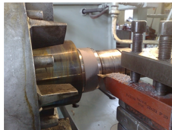
Processing of Belzona 1111 product
