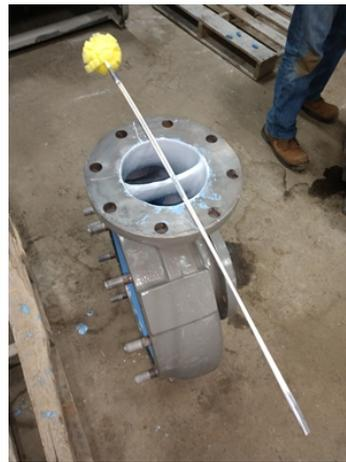
Applying the second coat of Belzona 1341.
