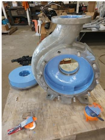
First coat of Belzona 1341 applied.
