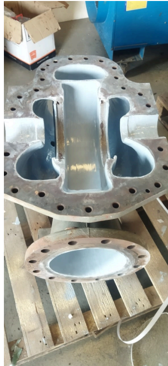
Pump after rebuilding and coating
