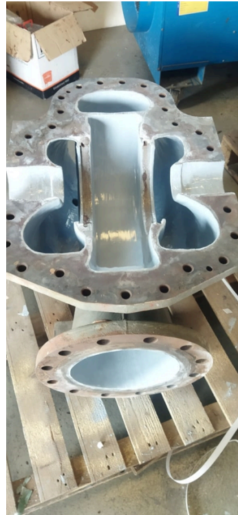
Pump after rebuilding and coating
