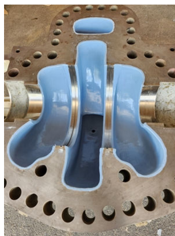
Pump casing protected with Belzona pump coating
