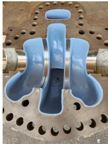
Pitting damage on the pump casing
