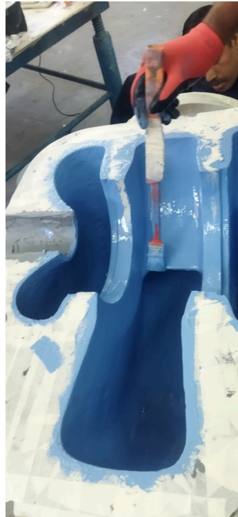
Coating application to the cutwater
