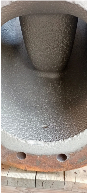
Pitting damage appeared after blasting
