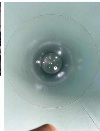
Internal reactor body before coating
