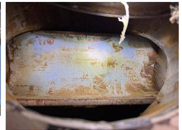
1 year on and the coating is still perfect, doing exactly as intended by avoiding build up of material and allowing the rotor to perform at full efficiency, whilst protecting against erosion
