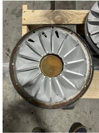
Area rebuilt with Belzona 1111 and protected with Belzona 1331.
