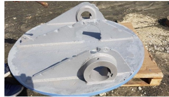
Belzona 1111 (Super Metal) rebuilt the damaged metal surface
