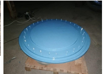
Valve coated with Belzona 1341 (Supermetalgilde)
