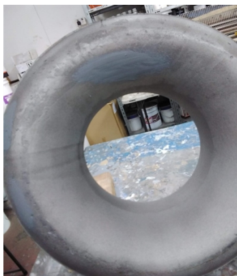
Pump housing abrasive blasted and Belzona paste grade metal utilised to repair erosion.
