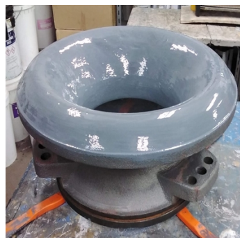
First coat of Belzona 1321 applied.
