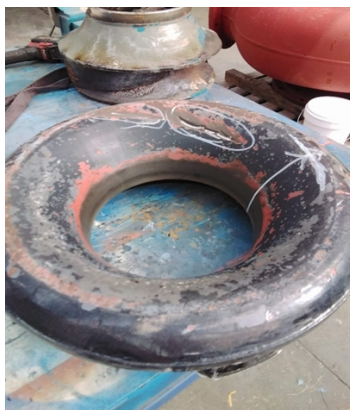
Damaged pump housing.
