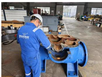
Degreasing and chamfering pump casing surface
