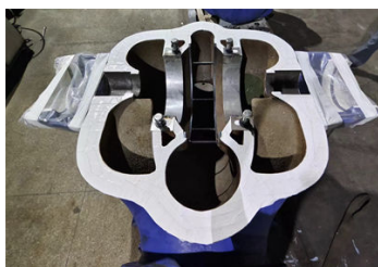
Protection of matching surface before surface preparation
