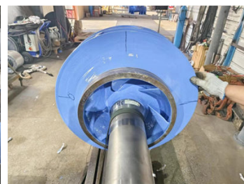
Dynamic balancing test after the impeller is coated with Belzona 1341
