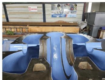
2 coatings of Belzona 1341 completed
