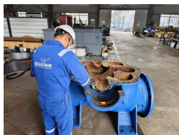
Degreasing and chamfering pump casing surface
