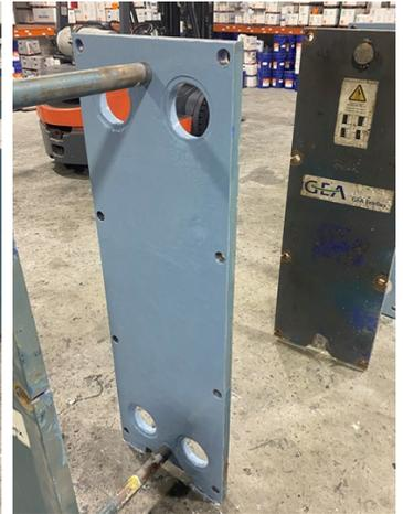
Areas to be rebuilt/coated were checked for chlorides, chlorides were neutralized to acceptable levels, units were blasted and profile checked as per product manufactures recommendations.
