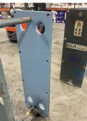
Areas to be rebuilt/coated were checked for chlorides, chlorides were neutralized to acceptable levels, units were blasted and profile checked as per product manufactures recommendations.
