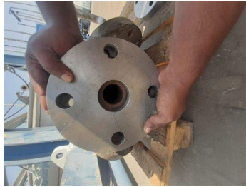
Forming technique was used to rebuild the flange face
