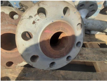
Worn-out flange face need repair
