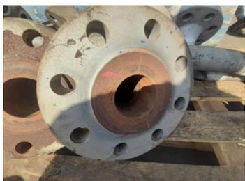
Worn-out flange face need repair
