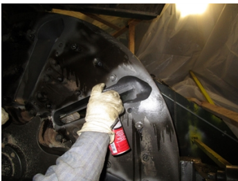
Pockets grit blasted and being washed with solvent.
