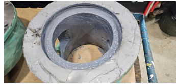
Lined with Belzona 1321
