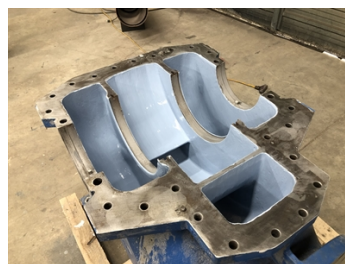
Finished application with the wear rings rebuilt and the pump casing coated with Belzona 1341N (Supermetalglide).
