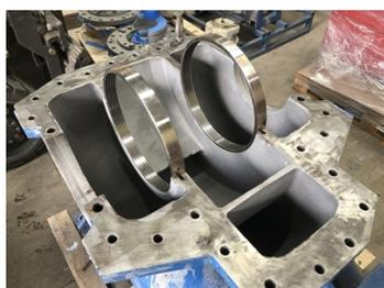
Pump grit blasted and new wear rings positioned.
