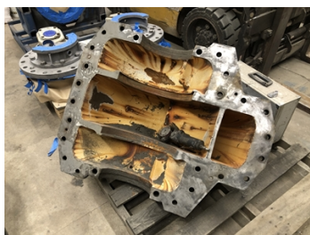
Condition of pump casing when pulled from service.
