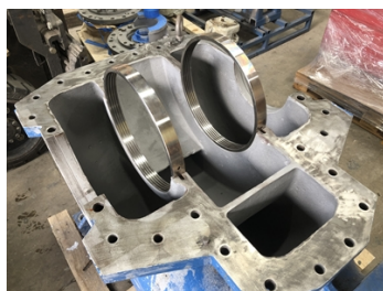
Pump grit blasted and new wear rings positioned.
