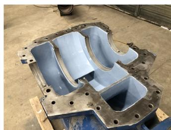
Finished application with the wear rings rebuilt and the pump casing coated with Belzona 1341N (Supermetalglide).
