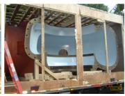
Applicator checking millage of Finished application, ready to close up the shipping crate and ship on to the customer.
