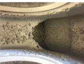
Cutwater was severely eroded. Picture shows completed
