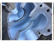
Picture shows completed application of Belzona 1341 (Supermetalglide) on the top half of the casing.
