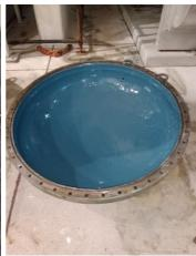
Rebuilding completed Belzona 1121.
