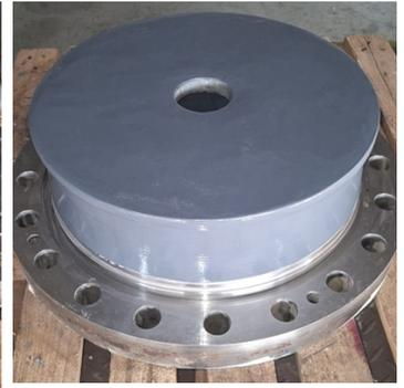
Final equipment after the Belzona 1321 application.
