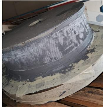
During the rebuilding works using Belzona 1121.
