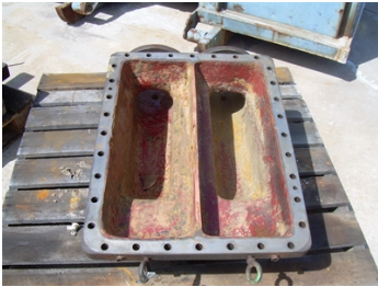
Overview of damaged hydrogen cooler head
