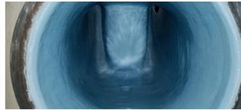
Pump component coated with Belzona 1341N
