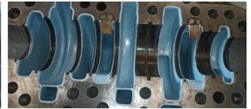
Pit filling with Belzona 1111 and coated with Belzona 1341N for the pump
