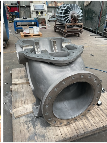
Pump casing abrasive blasted, ready for Belzona coating.
