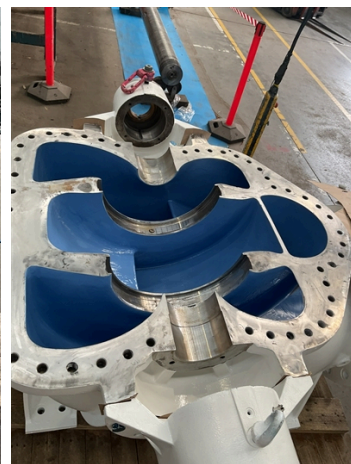
Belzona 1341 (Supermetalgilde) coating carried out.
