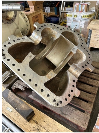
Internal split case pump prior to application
