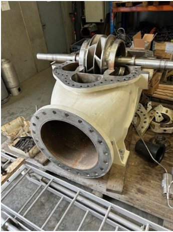
Split case pump prior to application.
