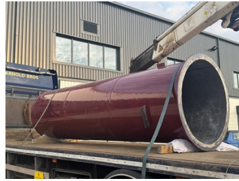
Internal lead lined bund
