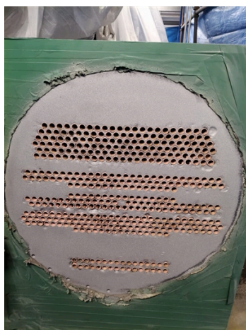
Tubesheet face after blasting
