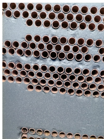
After blasting, significant metal loss was evident on the tubesheet face, requiring rebuilding with Belzona 1111
