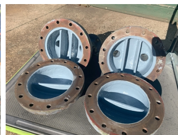
End covers completed with second coat Belzona 1391T Blue
