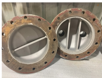
End covers were blasted for further repair steps
