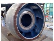
station's seawater intake pump cleaning with Belzona 9111. diffuser bowl and vanes from prolonged marine exposure is undermining efficiency, reliability, and structural integrity.
