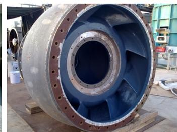
Extensive corrosion in a power station's seawater intake pump diffuser bowl and vanes from prolonged marine exposure is undermining efficiency, reliability, and structural integrity.
