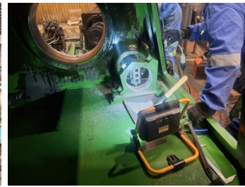
Surface machining after application of Belzona 1111
