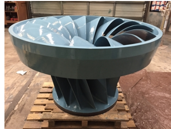
Coated with Belzona 1341
