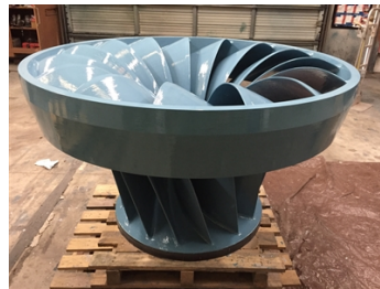
Coated with Belzona 1341
