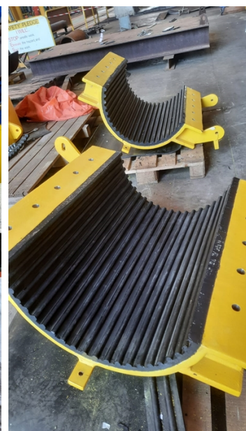
Completed Bonding Application
