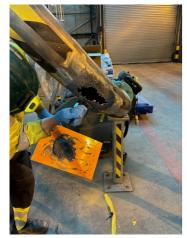
Pipe showing the large hole caused by sliding abrasion.
