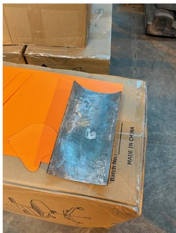
The Steel patch after surface preparation both sides, which is going to be bonded over the large elbow hole.
