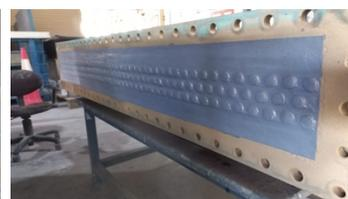
The heat exchanger tube sheet and cover suffered from metal loss and severe pitting as a result of erosion and corrosion.
