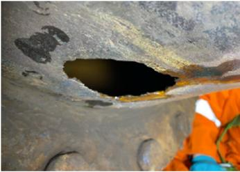
Through wall defect on pipe due to severe corrosion
