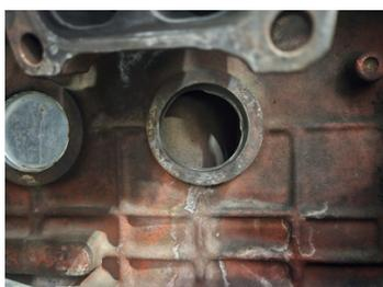
Engine block area with the freeze plug removed, exposing the internal cavity before repair.
