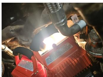
Controlled heat being applied to the engine block area using portable lamps to ensure proper curing of the repair material.
