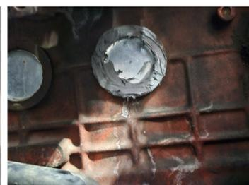
Freeze plug installed and sealed with epoxy compound after completing the engine block repair.
