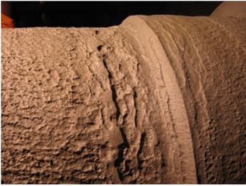
Severe Pitting Corrosion
