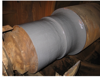
Belzona 1321 brush applied
