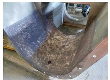
The new fabrication, following grit blasting to a profile 75 microns and a minimum of Swedish Standard SA2.5
