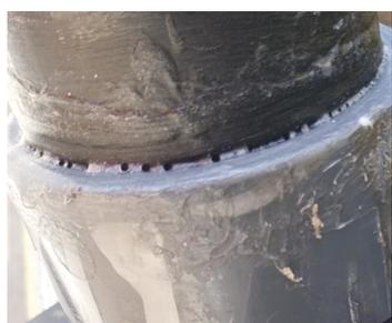
Showing porosity to glued collar, still allowing system pressure drop
