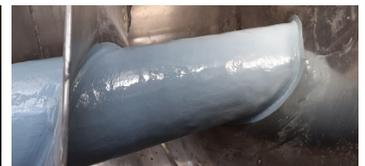
Wet pulp screw conveyor was suffering from localised erosion and scoring
