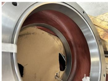
The pumps are grit blasted to a minimum surface profile
