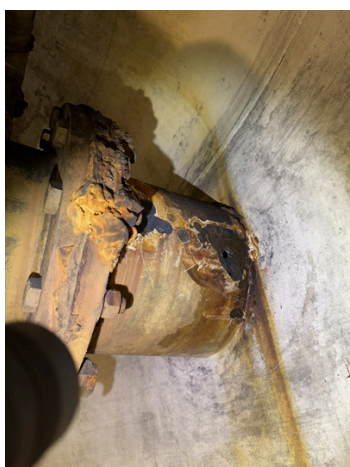
Problematic area showing the through wall defect
