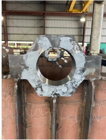
Holes filled with Belzona 1161 by injection.
