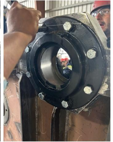
Bearing casing fit-tested for installation.
