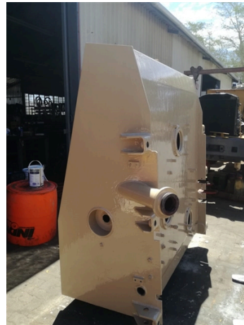
Second coat with Belzona 5811
