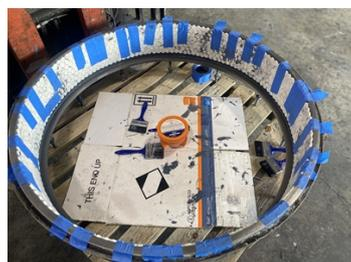
Applying Belzona 9811 alumina tiles
