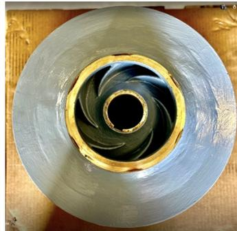
Top view of the repair using Belzona 1111 and brass plate
